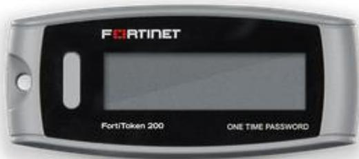
The button to the left hand side of the screen, push the button to display the current one time passcode. The number on the token changes every minute and the dashes on the left hand side are an indication of the remaining time that the current token has. The more bars, the longer that the code will be valid for.
