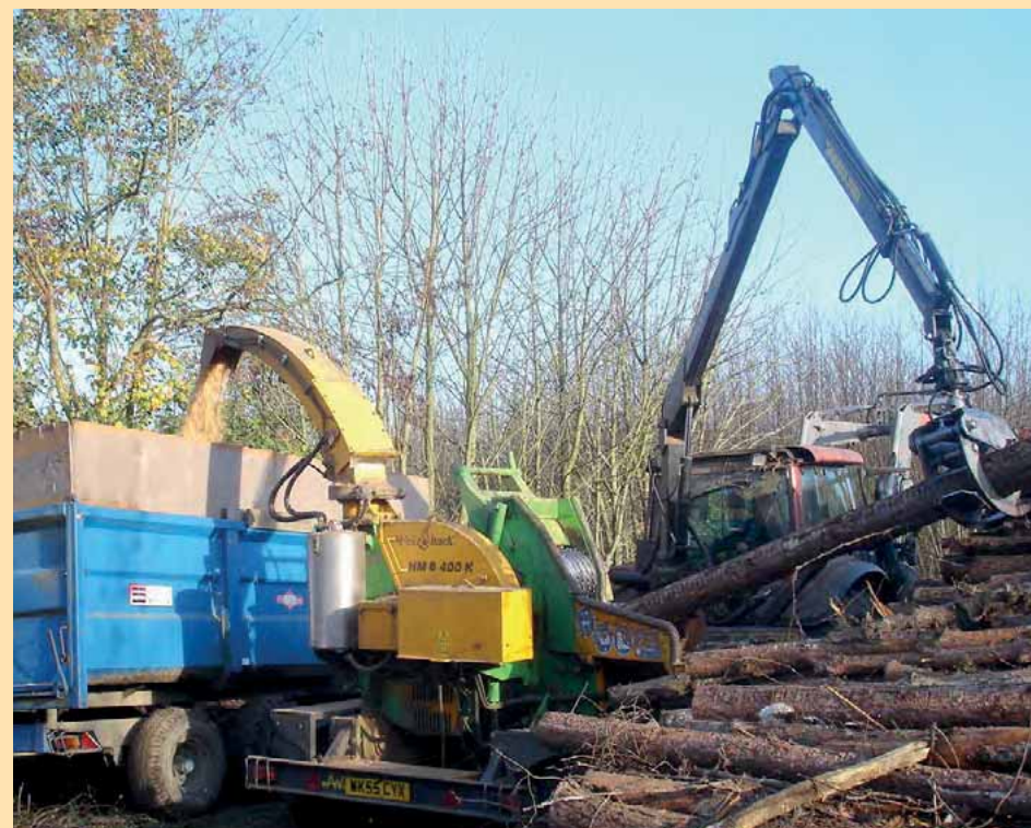
Wood chipping in action. The woodland resource provides an excellent opportunity for biomass energy in the form of wood chip.
