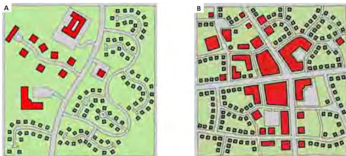
Figure 11.2 - Car dependent (A) versus walkable street layouts (B)
