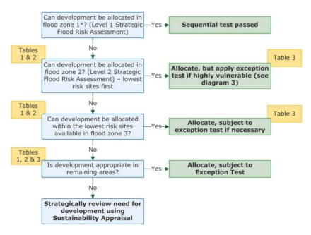
Figure 1: NPPG Flood and Coastal Change process for applying the Sequential Test
