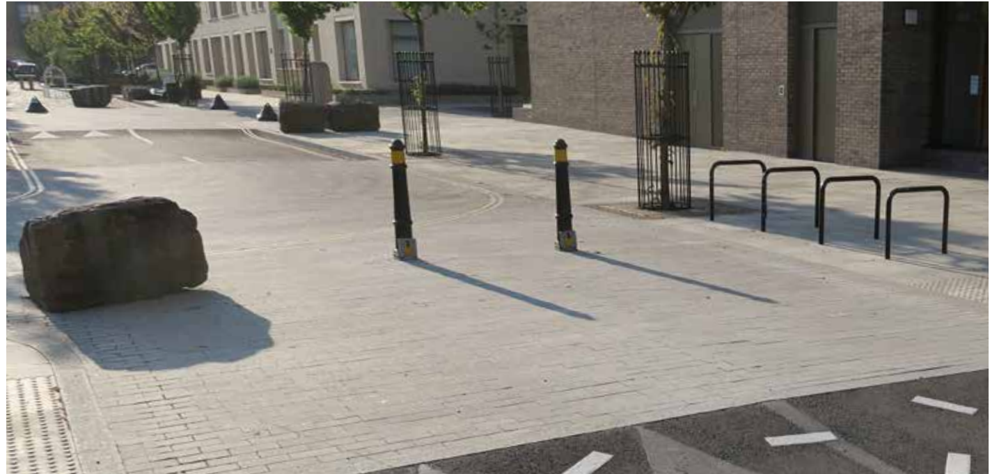
Figure 30: Collapsible bollards can be used to enable access to pedestrians and cyclists while retaining vehicle access for local residents, businesses, and emergency services only.
